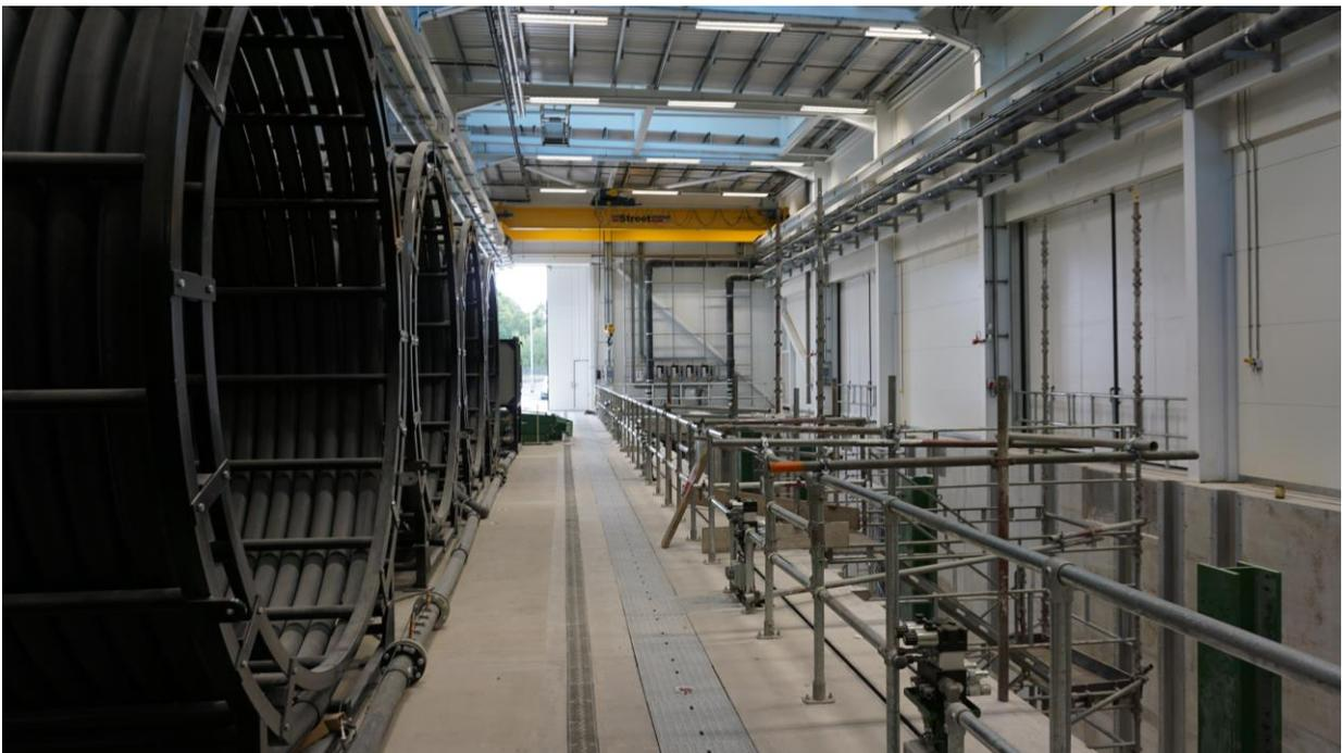
Full scale pipe loops for transient testing
