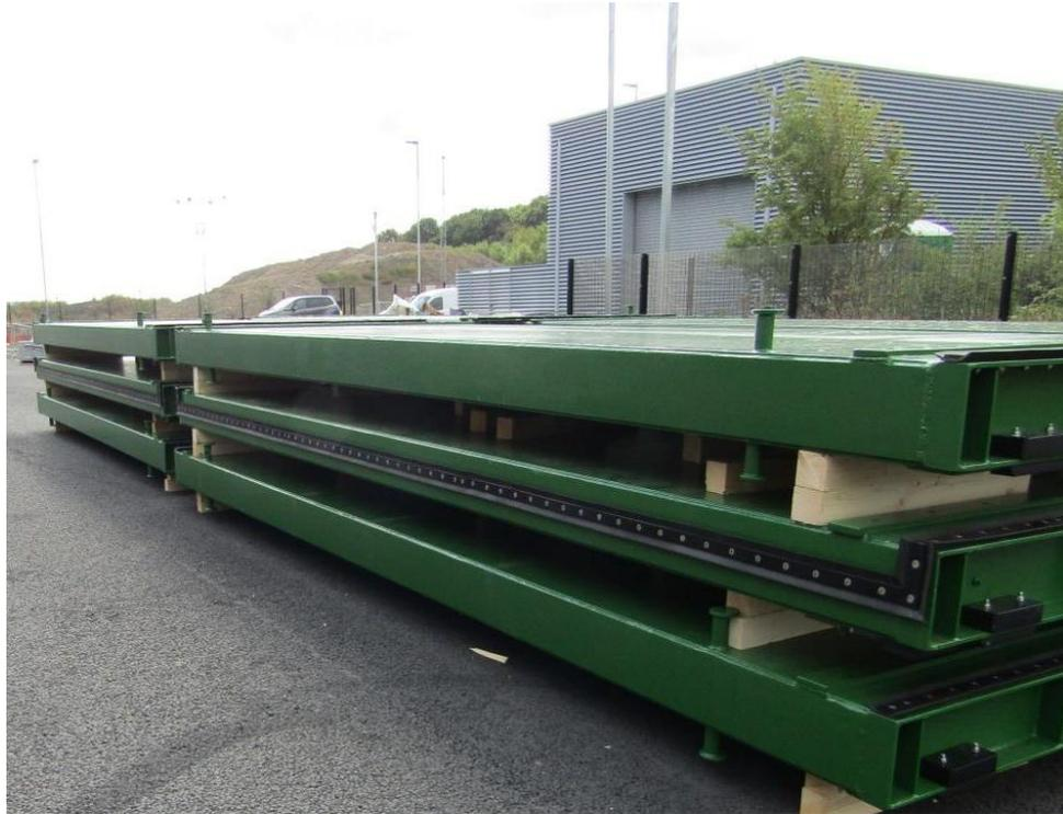
Stop logs used to divide testing tank
