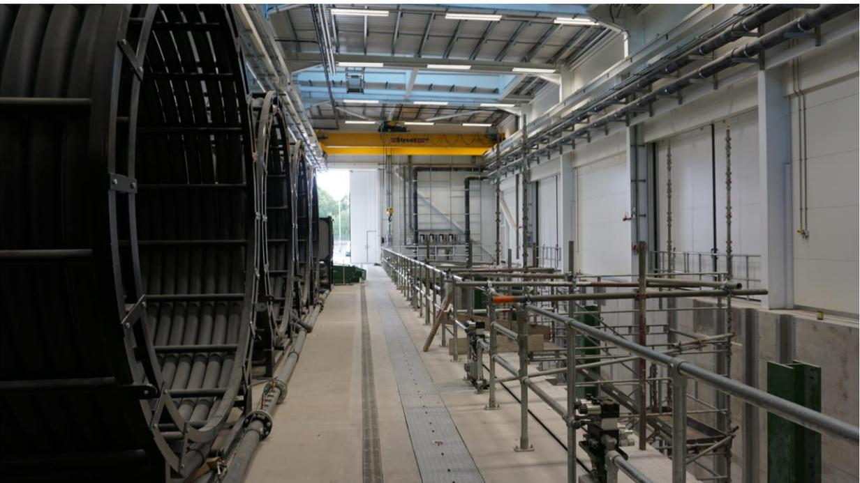
Full scale pipe loops for transient testing
